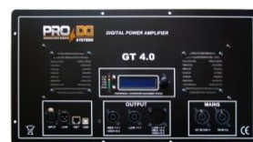
GT 4.0 1 canal / channel 2500 W graves / LF. 1 canal / channel 900 W medios / MF. 1 canal / channel 900 W agudos / HF.
